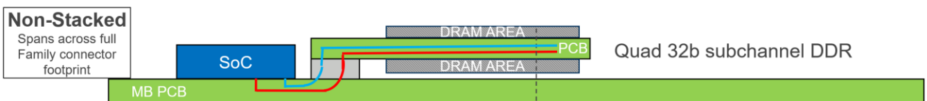
Figure 4 — Mounting of a Dual-channel CAMM2 with DDR5 DRAM
